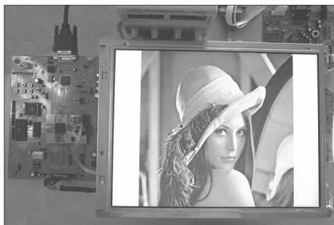
Figure 4. Implementation of image resizing algorithms in FPGA
