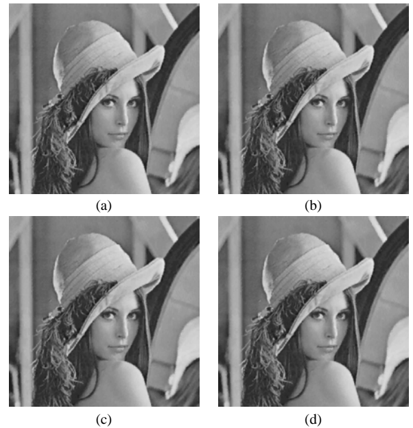
Fig. 8. Results of the decompressed images. (a) T = 16 , C_R = 17.241 , PSNR = 30.46 dB, SSIM = 0.9206, (b) T = 24 , C_R = 18.657 , PSNR = 30.51 dB, SSIM = 0.9297 (c) T = 28 , C_R = 19.083 , PSNR = 30.53 dB, SSIM = 0.9348 (d) T = 36 , C_R = 19.802 , PSNR = 30.57 dB, SSIM = 0.9353.
