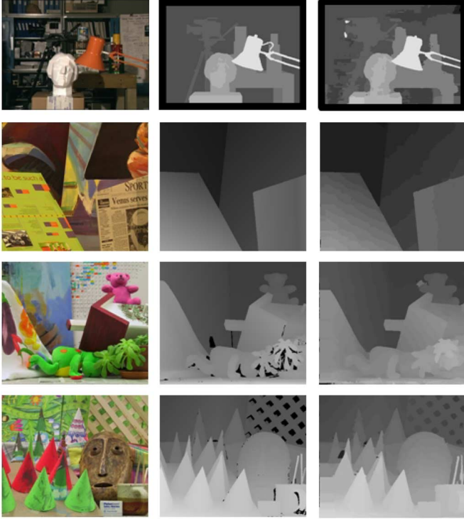
Fig. 13. Disparity maps for the “Tsukuba”, “Venus”, “Teddy” and “Cones”. Centered column shows ground truth disparity map and right-most column shows the disparity map from the proposed algorithm.
