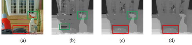
Fig. 5. Disparity maps on “Laundry” computed by different similarity measures. (a) Left image. (b) Color. (c) Combination of color and census. (d) Combination of color, census, and gradient.
